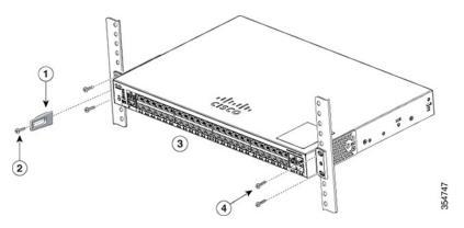
Due to design differences, some of the mounting brackets will attach such that the switch will protrude about an inch from the mounting surface.
