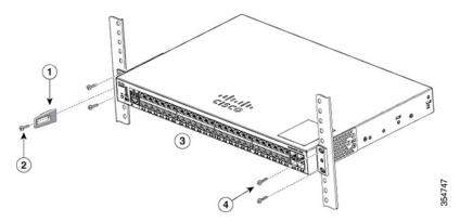
Due to design differences, some of the mounting brackets will attach such that the switch will protrude about an inch from the mounting surface.
